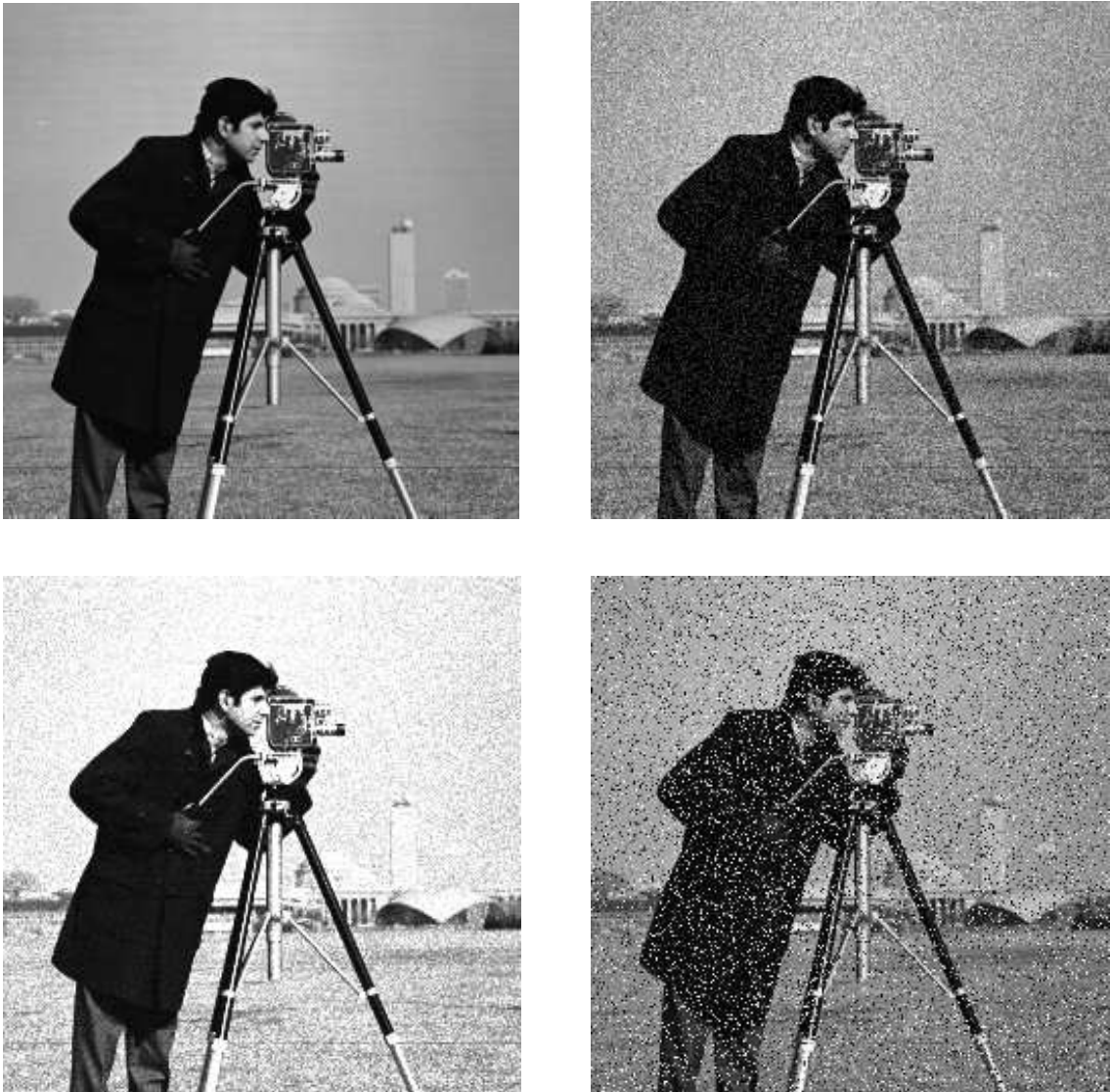
Figure 2.7: Different types of noise: (a) original image; (b) additive noise; (c) multiplicative noise; (d) impulse noise.
