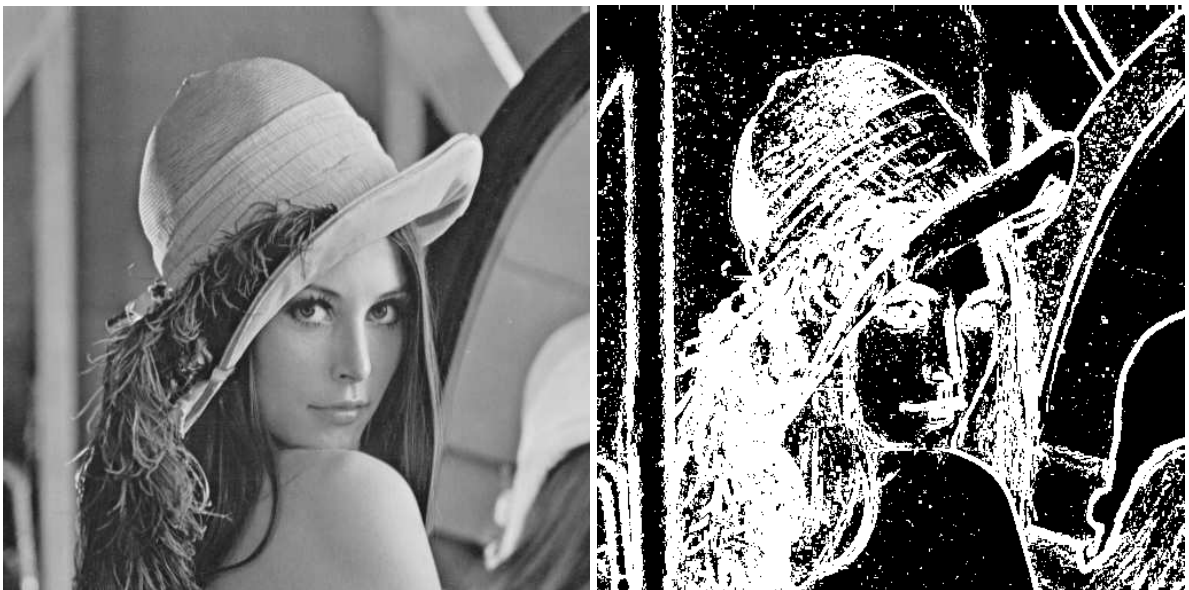
Figure 6.7: (a) original lenna ; (b) classification into smooth (black) and shaped (white) feature points.
