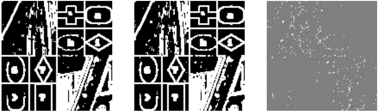
Figure 5.22: Model order selection when \sigma = 5 , black denotes k = 1 , white k = 2 : (a) Pseudo-MML; (b) MML; (c) difference: white shows where MML chose k = 2 over Pseudo-MML's k = 1 .
