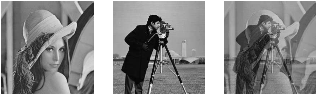
Figure 2.5: Alpha-blending example: (a) first image; (b) second image; (c) blended image using \alpha = 0.5 .
