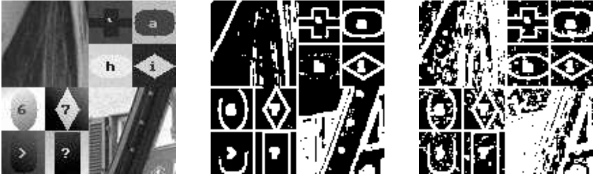
Figure 5.16: (a) noisy \sigma = 5 middle section of montage ; (b) FUELS model selection; (c) Pseudo-MML model selection. Black denotes k = 1 and white k = 2 .
