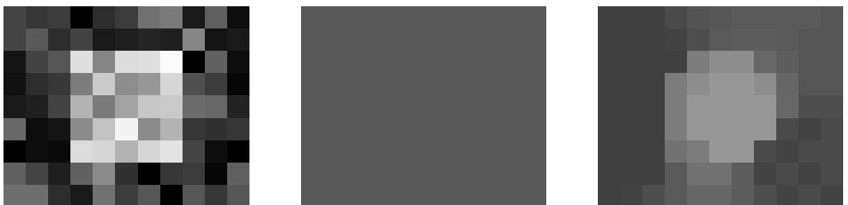
Figure 4.38: Iterating 100 times: (a) noisy \sigma = 40 square; (b) 3 \times 3 local segmentation assuming \sigma = 40 ; (c) 3 \times 3 median filtered.
