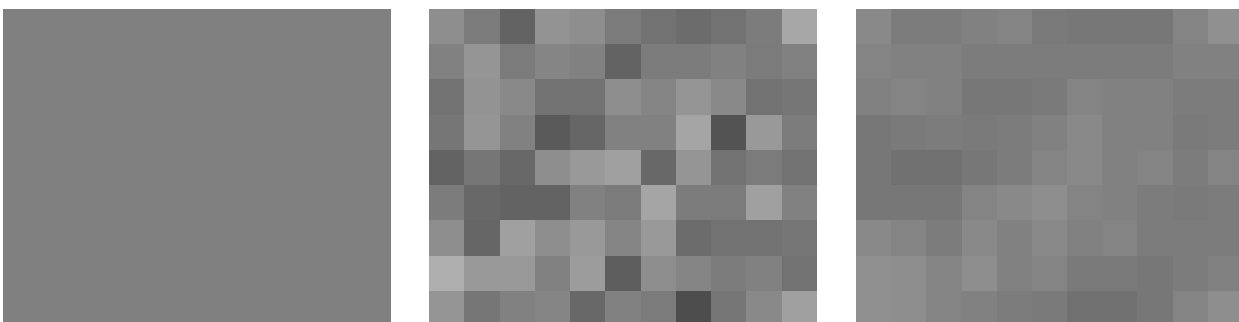
Figure 3.12: Application of the 3 \times 3 box filter: (a) original; (b) noisy; (c) filtered.
